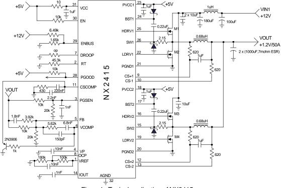
Figure1 - Typical application of NX2415
