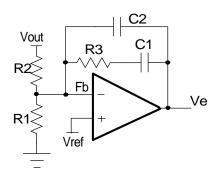
Figure 4 - Type II compensator
