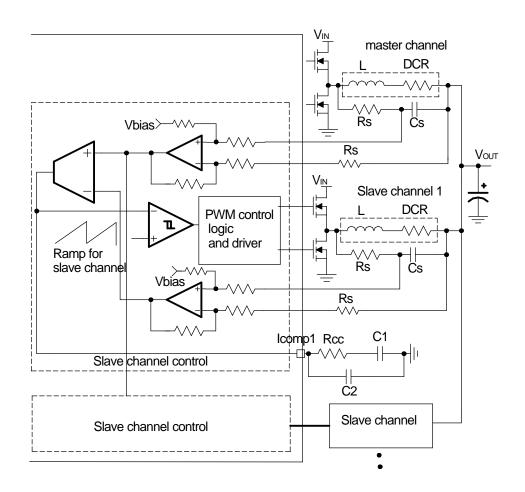
Figure 7 - Function diagram of current loop
