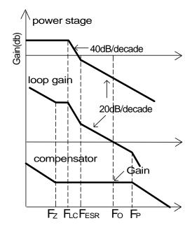
Figure 5 - Bode plot of Type II compensator
