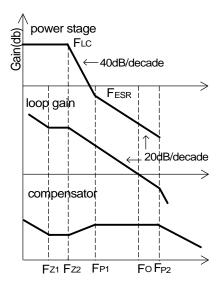
Figure 3 - Bode plot of Type III compensator
