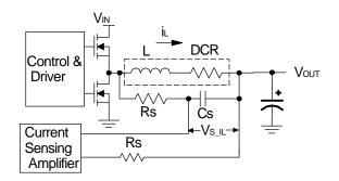
Figure 8 - Inductor current sensing using RC network.
