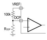
Figure 12 - Over current protection
