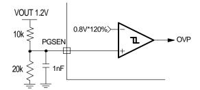
Figure 14 - Over voltage protection
