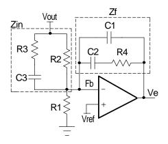
Figure 2 - Type III compensator
