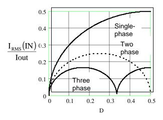
Figure 15 - Normalized input RMS current vs. duty cycle.
