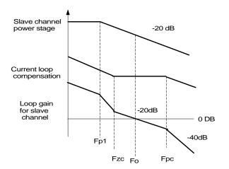
Figure 10 - Bode plot of current loop
