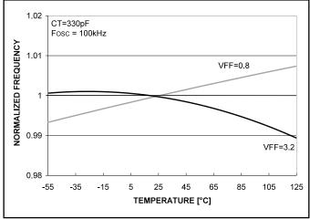
Figure 4. Oscillator frequency vs. temperature.
