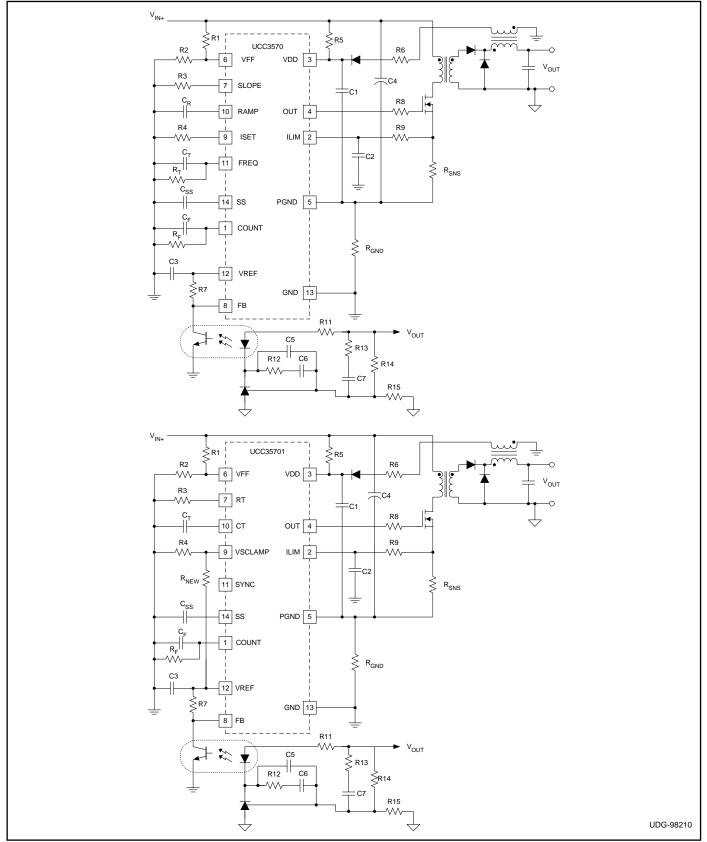
Figure 6. Single-ended forward circuit comparison between UCC3750 and UCC37501.
