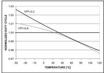
Figure 5. Normalized maximum duty cycle vs. temperature.
