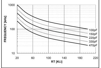
Figure 3. Oscillator frequency vs. RT and CT.
