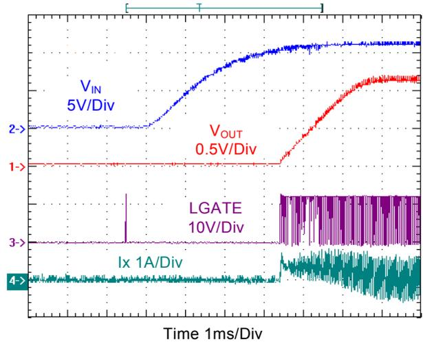
Figure 3. Softstart where  $V_{IN}$  does not Present Initially.
