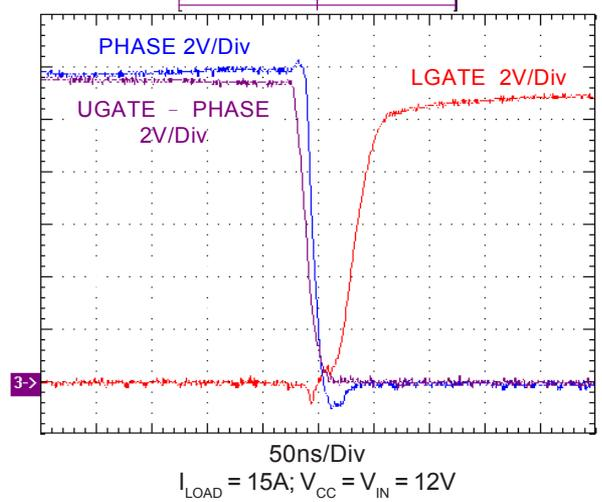
**UGATE Turn Off Waveforms**
