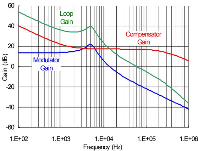
Figure 11. Gain vs. Frequency for the Design Example.
