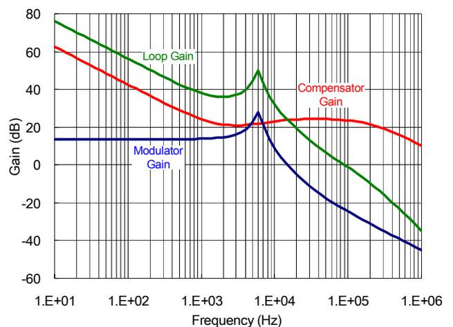
Figure 14. Frequency Response of Type III Compensation.
