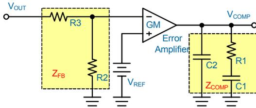
Figure 7. Type II Compensation Network Using OTA.
