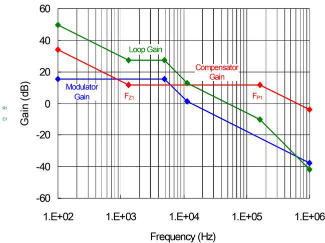
Figure 8. Frequency Response of Type II Compensation.
