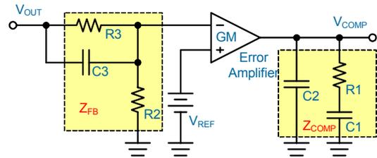
Figure 12. Type III Compensation Network.
