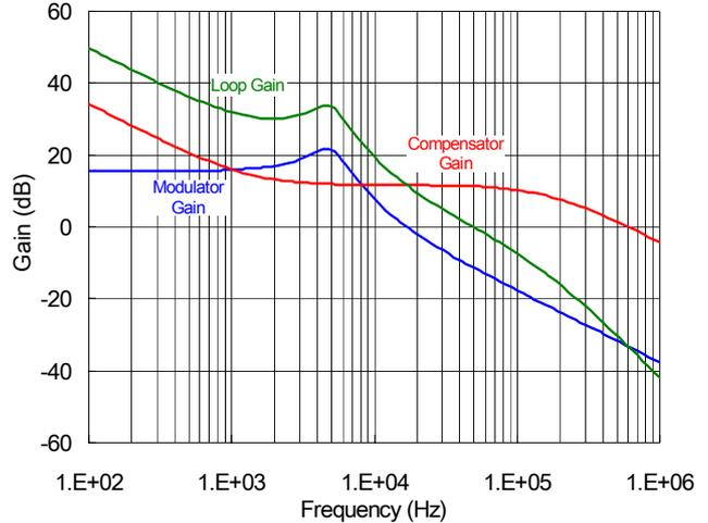
Figure 9. Frequency Response of Type II Compensation.
