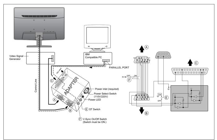
Figure 1. Cable Connection
