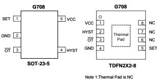
Note 1: I nermal Pad is NC Note 2:Connect Thermal Pad and pin 6,7,8 to heat source by PCB copper for good heat conduction.
