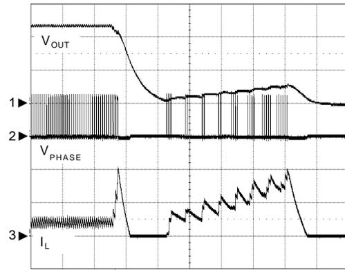
CH1:  $V_{OUT}$ , 500mV/Div
