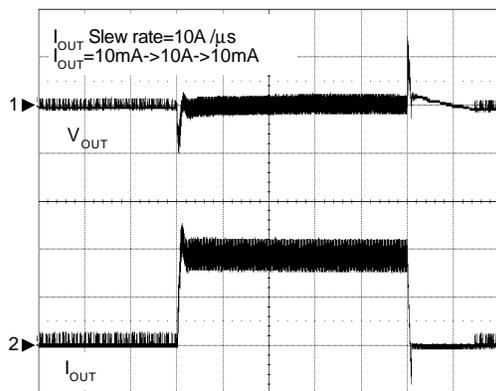
CH1:  $V_{OUT}$ , 50mV/Div
