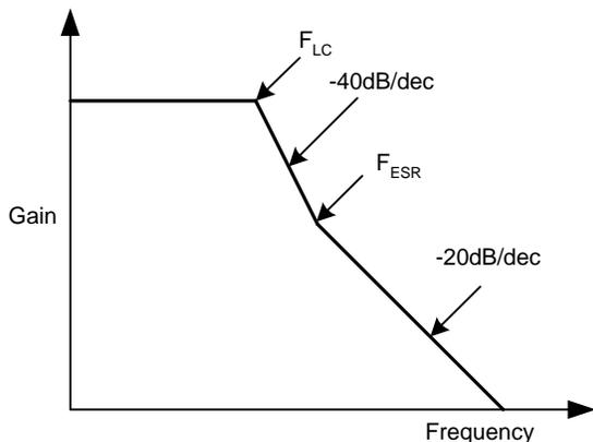
Figure 3. The LC Filter Gain & Frequency
