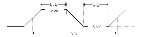
Figure 11-1. Clock Input Timings
