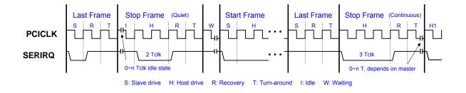
Figure 9-2. Stop Frame Timing
