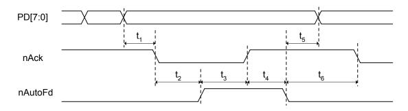
Figure 11-10. ECP Parallel Port Backward Timings
