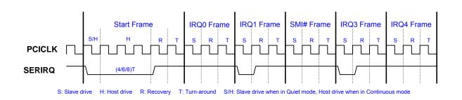
Figure 9-1. Start Frame Timing
