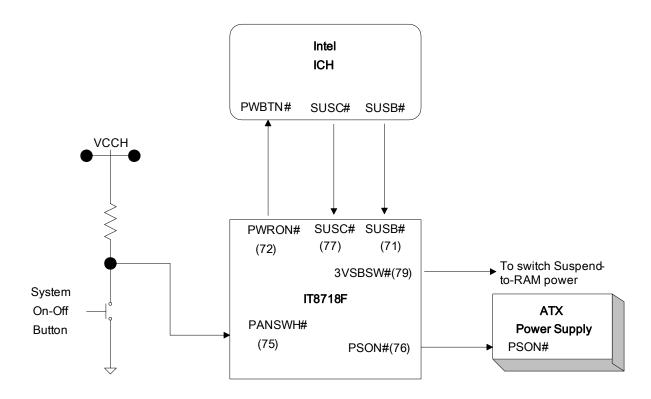
Figure 7-1. IT8718F Special Applications Circuitry for Intel ICH This page is intentionally left blank.
