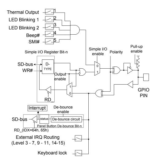
Figure 9-3. General Logic of GPIO Function
