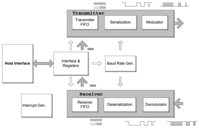
Figure 9-8. CIR Block Diagram
