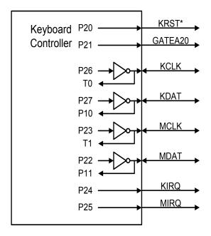
Figure 9-7. Keyboard and Mouse Interface
