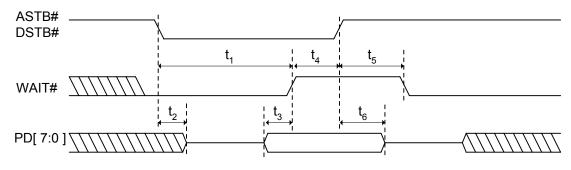
Figure 11-8. EPP Address or Data Read Cycle Timings
